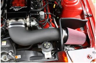
Plug in MAF sensor and supplied PCV hose and you're DONE! Do not tighten clamps more then finger tight!!
