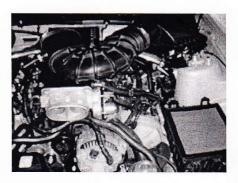
**Step 2:** Remove the drive belt and alternator.
