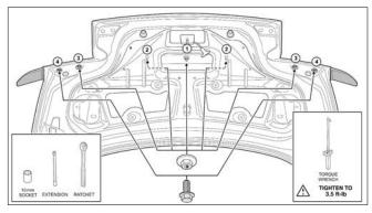
23. Re-install the two (2) OE rubber hole plugs removed in step 3. Install four (4) new 1.0" rubber holes plugs into the access holes drilled in Step 7.
