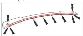
19. Install the rear spoiler through the holes drilled into the trunk lid. Do not allow the exposed double-sided tape to adhere to the sheet metal until you have confirmed the spoiler is centered, then push down.
