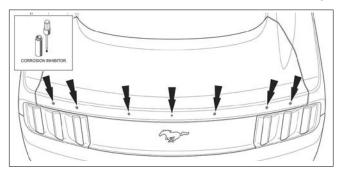
18. Prepare rear spoiler for installation. Peel back 2.0" (50.0 mm) of each tape liner and secure each liner to the outer surface of the rear spoiler using masking tape.
