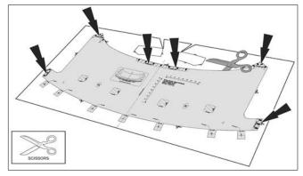
10. Install the trunk lid outer sheet metal drill template. With the trunk lid closed, align the large outer drill template onto the outer sheet metal of the trunk lid as shown. Secure template to trunk lid with masking tape.
