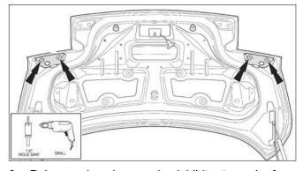
8. Deburr and apply corrosion inhibitor to each of the four (4) 1.0" access holes. Allow to dry.
