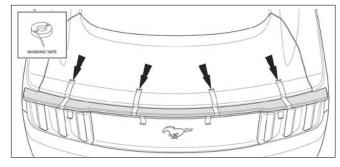
13. Open the trunk lid and inspect each of the seven (7) mounting holes. Confirm that the rear spoiler fasteners are properly aligned with the holes drilled in the trunk lid outer sheet metal.
