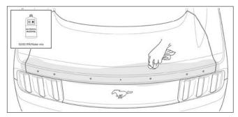
17. Deburr and apply corrosion inhibitor to all the holes drilled in the outer sheet metal. Allow to dry.
