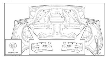
7. Create four (4) access holes in the trunk's inner sheet metal by center punching four (4) hole locations, two (2) per side. Drill each center punched location with a 1/8" drill bit. Enlarge each 1/8" hole with a 1.0" hole saw.
