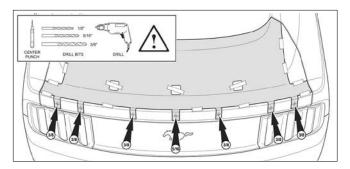
12. Test fit the rear spoiler. Align the five (5) studs on the rear spoiler through the holes drilled into the trunk lid. Secure the rear spoiler to the trunk lid with masking tape.
