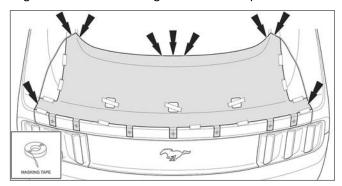
11. Drill seven (7) rear spoiler mounting holes. Center punch the seven (7) hole locations indicated on the template. Drill each center punch location with a 1/8" drill bit. Enlarge each 1/8" hole to the size indicated on the template. Note that the center hole should be enlarged to 5/16" while the other six (6) holes should be enlarged to 3/8".
