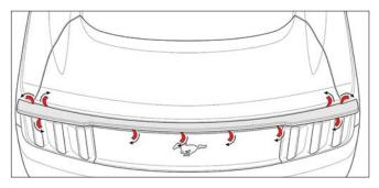
21. Using a rubber roller or the palm of your hand, apply 15 ft-lb of force to the tape area to 'wet-out' the tape. Start from the center of vehicle and work outwards.
