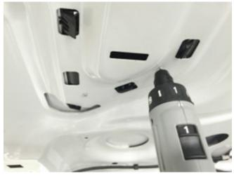
11. Reinstall the factory black plastic piece with the two (2) nuts that were removed in step 3. Torque them to 1.4 Nm.
