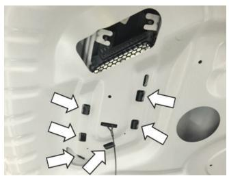
6. Cut out the drill templates from the last page of this instruction manual, tape them in place as shown below and then mark the two (2) drill holes with a center punch.
