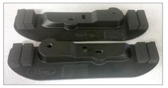
9. Remove the two (2) studs from the stock heat extractors and install them on the ROUSH heat extractors.
