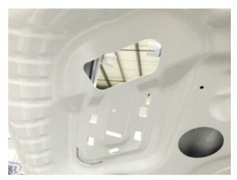
5. Release six (6) clips on each factory heat extractor and remove them from the vehicle.
