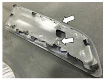
10. Install the ROUSH heat extractors by clipping them into the factory slots and installing two (2) T10 screws (P/N: 96817A350) in the holes that were drilled in step 6. Torque the screws to 0.4 Nm.
