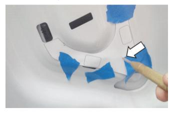
Drill each hole with a 1/8" bit. After the holes are drilled, apply commercially available clear coat (Motorcraft Part Number: PM-19500-6000) to the exposed metal so that it does not rust.
