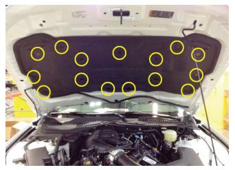
2. Remove the two (2) adhesive pads that retain the cables for each factory heat extractor.
