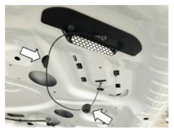
3. Remove two (2) 9 mm nuts at the bottom front edge of each factory heat extractor.
