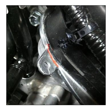
Step 2 – Retain the harness and hose aside and using a suitable cutting tool (cut off wheel, air saw, etc.) remove the tab from the front cover so it is flush with the edge of the cam cover. Use caution to not cut or damage any of the surrounding components.
