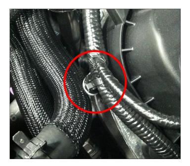
Step 1 – Locate the wiring retention tab on the front cover in front of the driver side cam cover. Using a trim tool, remove the wire harness retainer from the tab.
