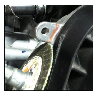
Step 3 – Using a suitable grinding tool (Air Grinder, hand file) remove any burrs and sharp edges. Remove the wiring harness push pin retainer from the wire harness.
