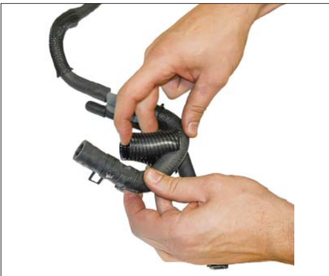
14. Loosen the clamp and rotate the curved hose (hose 4) end 180 degrees. Reinstall the clamp.
