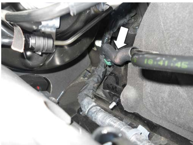
Disconnect green quick connect fitting
