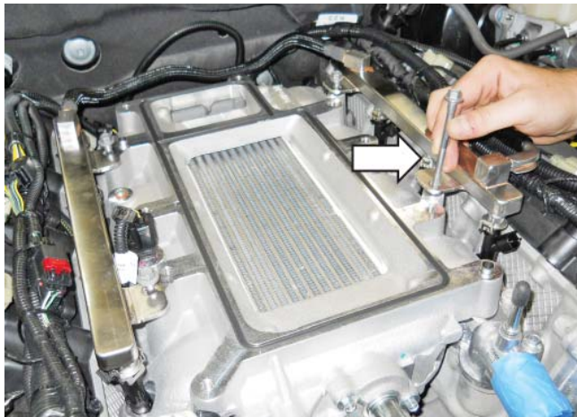
8. Connect the eight (8) fuel injector electrical connectors.
