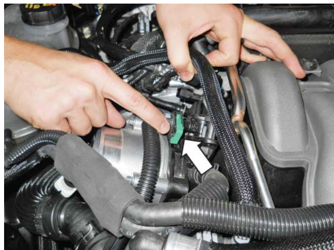
EECPV tube quick connector with green lock
