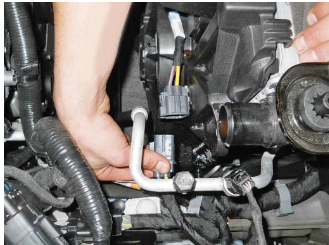
Fan shroud electrical connector
