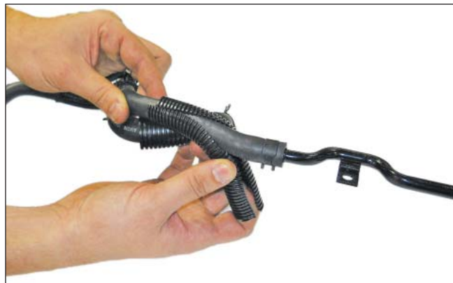
9. Release the clamp and separate Section B, hose 2, from the steel tube.
