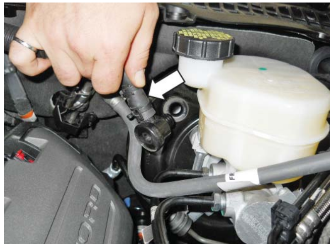
33. Remove the brake boost vacuum hose/line from the vehicle and set it aside. This line will be modified.
