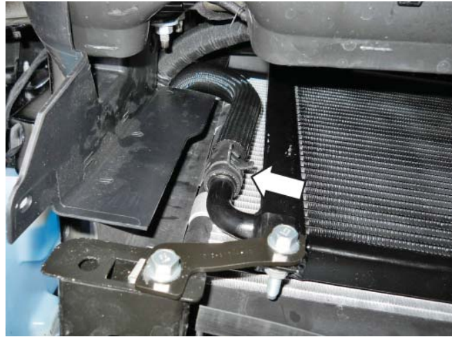
Pump hose to LTR connection
