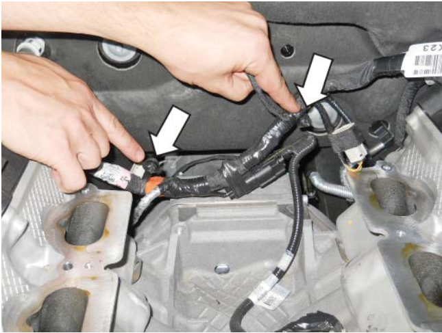
Pin retainers on harness
