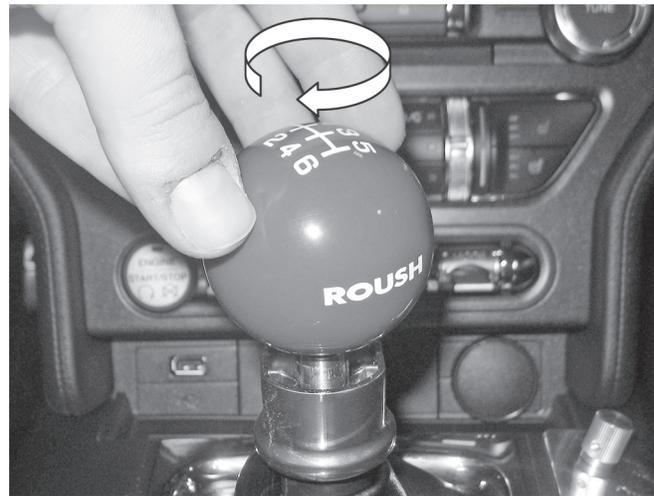
3. Screw the shift ball down until the bottom of the ball sits lower than the top of the positive lockout, and then continue to turn clockwise until the shift pattern on the top of the ball rests in the desired position.
