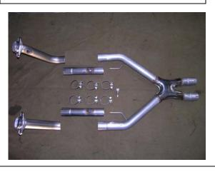
Note: anti-seize should be applied to all fastener threads and pipe slip joints
