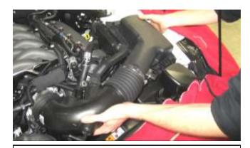
f. Pull the intake duct off the throttle body and lift out the factory intake assembly including the sound tube.
