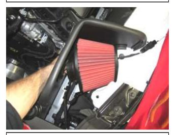
h. Install remaining hose clamp on the filter and lower the filter into the vehicle as shown and twist into place once the flange has started on the end of the tube.
