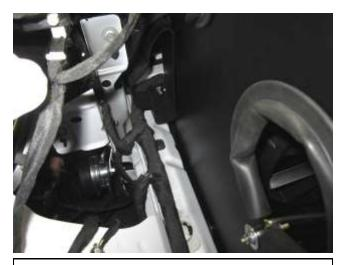
b. Lower the heat shield into the vehicle taking care to align the shield between the fresh air supply and the radiator as shown above.
