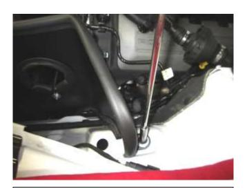
d. Reinstall the factory fastener at the upper mounting tab location of the heat shield.
