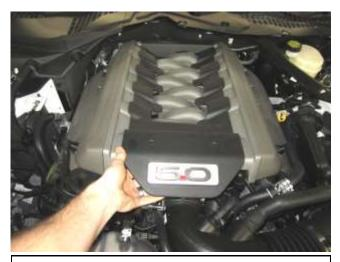
a. Lift up firmly on engine cover front and back to disengage and remove the engine cover.
