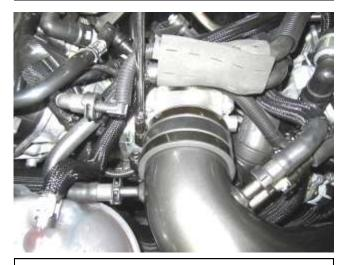
g. Lower the tube into the vehicle aligning the filter end in the heat shield first and then slipping the hose over the throttle body. Push on all lines as shown above until they click on securely. Ensure that wiring harness remains in front of the bracket on the bottom of the tube and reconnect to the MAF sensor.
