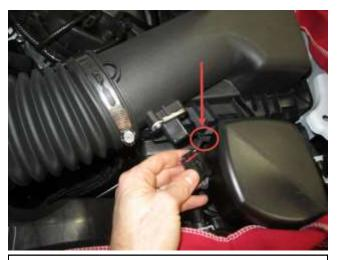
d. Disconnect MAF sensor wring and use needle nose pliers to pry the retaining clip out of the airbox (circled above). Remove the MAF sensor using the included TORX key and set aside.
