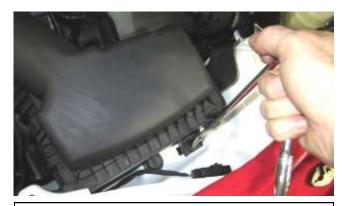
e. Remove the 10mm bolt securing the factory airbox. Ensure that the nut clip does not fall into the fender well.
