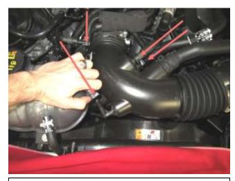
b. Release the three quick disconnect fittings from the factory intake duct and loosen its hose clamp at the throttle body.
