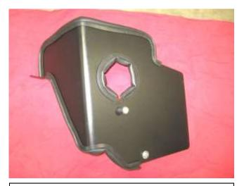
a. Assemble the heat shield according to the exploded view on page 2 of this document as shown including the edge trims & rubber mount below the intake tube hole.
