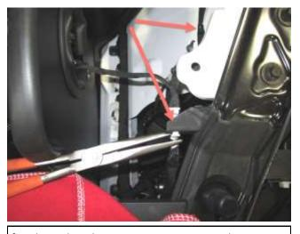
f. Release the other sensor wiring retaining clips. Pass the harness through the tube hole in the heat shield.
