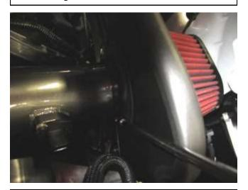
j. Slide filter clamp through the heat shield hole and tighten on the engine side of the shield ensuring that the clamp remains fully engaged on the filter.
