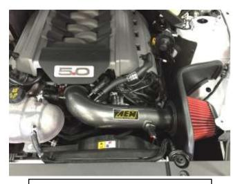
p. Finished installation of AEM Intake System.
