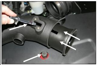
the MAF sensor. Next install the MAF sensor into the intake tube using two provided 8-32x3/8" screws (#14). **Do Not Use The Factory Screws!**
