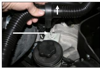
from the stud securing the power steering reservoir. Using a deep 10mm socket, remove the stud and save it for a possible optional install. See step #18.
