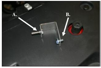
10.**A.**) Thread the 1/4-20 hex bolt (#15) into the resonator bracket (#22) and tighten as shown. **B.**) Slide the 6mmx12mm (#16) hex bolt thru one flat washer (#13) and into the hole in the resonator bracket.
