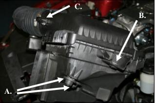
3. Grab the airbox and tube and roll it forward while lifting up to dislodge it from the intake scoop. Remove the assembly from the vehicle. A.) Remove the two factory grommets and then replace them back into the two holes in the inner fender. B.) Remove the steel sleeve and grommet and save for reinstallation later. C.) Using the provided #20 Torx bit, remove the two screws and the **MAF** sensor from the tube.
