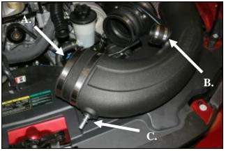
now. B.) Install the 1 3/4" coupler (#7) onto the intake tube using two #28 hose clamps (#18) as shown. Tighten only the clamp against the tube for now. C.) Install the provided grommet (#19) into the intake tube and then install the aluminum fitting (#21) into the grommet as shown.
