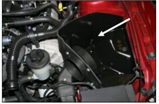
and towards the front. The last anchor nearest the MAF was removed in step #2 thru the steel sleeve and grommet and into the inner fender. Make sure that the wiring harness is not pinched under the CAD.
