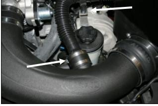
and then onto the throttlebody. Adjust for fit and then tighten all four hose clamps. Next, reinstall the factory clamp. Now "reseat" the resonator tube onto the bracket.
