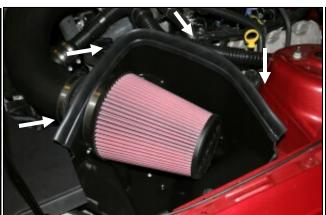
adapter and tighten the hose clamp. Next, install the connectors, cut the factory breather tube on each end just weatherstrip (#11) onto the top of the CAD as shown enough to remove the factory connectors. resonator tube into the 1 3/4" coupler and tighten the hose starting near the radiator and working your way towards the left fender.
