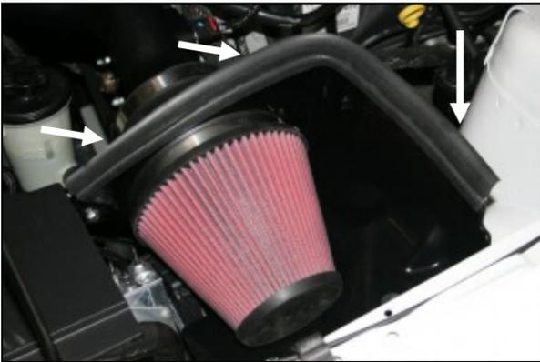
14. Install the Airaid Premium Filter (#1) onto the filter adapter as shown and tighten the clamp. Now install the supplied weather strip (#7) onto the top of the CAD as shown starting near the radiator and working towards the left fender.
