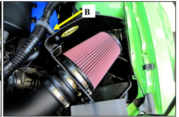
12. **A)** Install the Airaid Premium Filter onto the filter adapter and tighten the hose clamp. **B)** re install the Resonator tubing into the factory Stand off.
