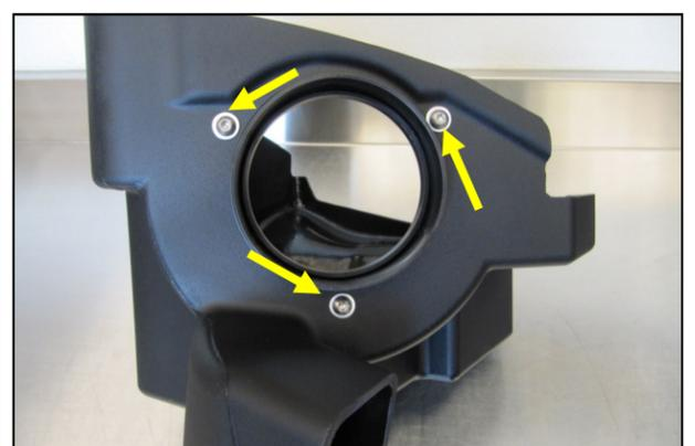
**4. Install the Grommets and Fittings into the Airaid intake tube A)** All models will require the use of the 5/8" Fitting (#19) and the 5/8" Grommet (#20). **B)** Automatic transmission equipped vehicles will also use the 3/8" Fitting (#18) and 3/8" Grommet (#21). Manual transmission vehicles will not need the 3/8" components and will use the Blind Grommet (#22).
