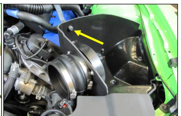
**7. Transfer the factory air box mounting grommets. A)** Locate and remove the Two Lower air box mounting grommets, and install them in the inner fender. **B)** Remove the Upper air box mounting grommet and steel sleeve, and re-install into the Airaid Cool Air Box
