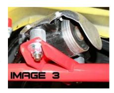
18. Due to production tolerance, an alignment is recommended after this installation.
