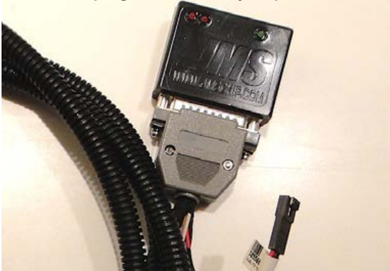
ID the Tip Sensor Connectors: Cable is labeled: TIP Three Wires
