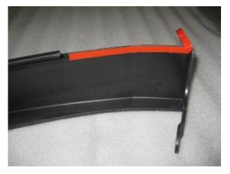
6. Install **Chin Spoiler**. Place Chin Spoiler on the Fascia, making sure the "pull tabs" are all accessible. Peel red backing and press Chin Spoiler firmly to activate adhesive.
