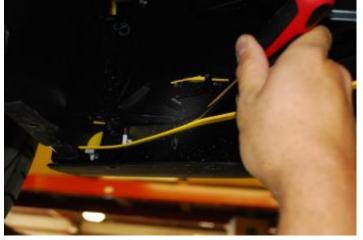
4. Remove "U" Clips from Fascia and Splash Guard. Note: Clips will NOT be reinstalled.
