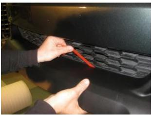
7. The retainers removed in step #3, are to be replaced with the new larger diameter Push Pins.
