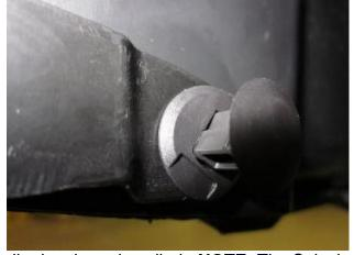
Picture below for reference, after the Outlaw Chin Spoiler has been installed. **NOTE:** The Splash Guard will rest on the Chin where the arrows are pointing.
