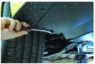
3. Remove the Performance Pack Chin Spoiler. Remove all the 7mm fasteners and push pin retainers. **Note:** The Factory Chin will NOT be reinstalled.
