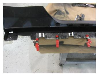
10. Using the holes in the Outlaw Rockers as drill guides, drill 3/16" holes as shown and install the supplied 3/16" rivets.
