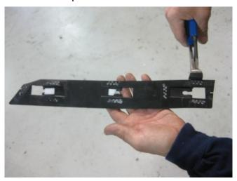
14. Clean the back side of the Outlaw Rockers, and the back side of the Bracket removed from factory rocker with the supplied Alcohol pack and allow to dry. Apply the supplied Adhesion Promoter to the same areas and allow to dry.
