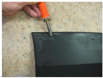
4. Remove the push pin retainer located at the rear of the Rocker. Remove (2) push pin retainers located at the front of the Rocker. Remove the (8) push pin retainers from the bottom of the Rocker. NOTE: Keep the factory retainers as they will be reused. Use a Panel Tool similar to picture below.
