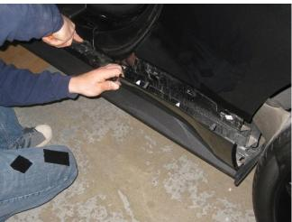
6. Remove Aero Deflector from stock Rocker. Remove the T-27 screws and "J" Clips (will be installed on your Outlaw Rocker).
