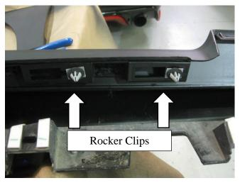
18. Install the Outlaw Rockers. Starting at the front, align the Rocker Clips and snap into place. Reinstall the Push Pin fasteners in the wheel openings and the underside.
