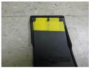
2. Assemble the Winglets to the Outlaw Rockers. <u>Note:</u> The Winglets are separate to make the painting process easier. The parts are pre-taped with 3M VHB tape. Remove the Masking tape from the back side of the Winglets, clean with the area with the supplied Alcohol Pack, and allow to dry. Apply the supplied Adhesion Promoter and allow to dry. Peel the red backing from the tape, use the alignment pins to locate the parts, and press the parts together firmly.
