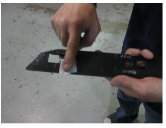
15. Apply the supplied 3M VHB tape to the back side of the Bracket as shown in picture below, cut to length with a razor blade.
