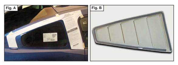
**Pre-fitting the Quarter Window Louvers:** Align the template with the factory bodyline on the top of the quarter panel and the painted edge behind the window molding **as shown in fig A**. Tape the template in place. The same template is used for both sides.
