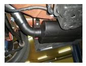
12) Place a 3" clamp onto the inlet pipes of the mufflers. Slide the hanger mounts removed in step 6 onto the new mufflers. Place the mufflers up into position and onto the over-axle pipes, and connect the rear hanger mounts to support. Secure the double hanger mounts back into position on the frame using the factory bolts.
