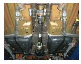
4) Use a 15mm socket to loosen the nuts on the clamped connections at the rear of the factory H-pipe and remove the intermediate pipes. Slip the pipes off and remove from the vehicle.
