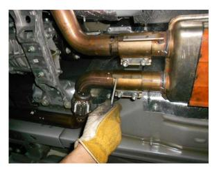
2) Support the center resonator with a stand, then loosen the four nuts and the two band clamp connections at the resonator inlet, use a screwdriver to pry up the clips on the clamp body to release the clip from the tab on the inlet pipes. Slide the clamp assemblies slightly back to clear the tabs.
