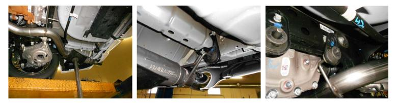
4) Place the right muffler assembly **#815430-387** up into position and slide the inlet completely onto the **26515S** mid pipe. Support the assembly with a stand and remount the rear hanger mount to the frame, tighten securely. Remount the front hanger to the cross member and tighten securely. Leave the clamp on the inlet loose for now. Repeat this step with muffler assembly **#815430-386** on the left side of the vehicle.
