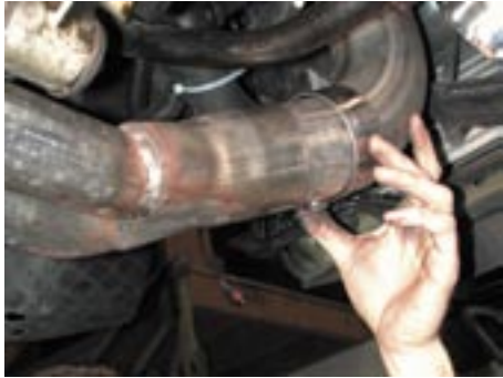
102. Hang double barrel pipe on rubber dog bone.
