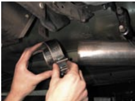
103. Install straight pipe or catalytic converter onto the double barrel. Again, slide clamp on first.
