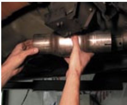
104. Install Y-pipe onto straight pipe or cat, sliding clamp on first. If desired, Install O2 sensors. If rear O2 sensors are to be used, extending the factory harness by cutting & soldering the wires will be necessary or buying o2 sensor extensions.
