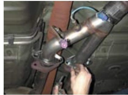
106. Position the entire exhaust system with about 1/2" clearance from other parts.
