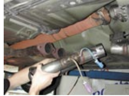
105. Bolt Y-pipe to mufflers.
