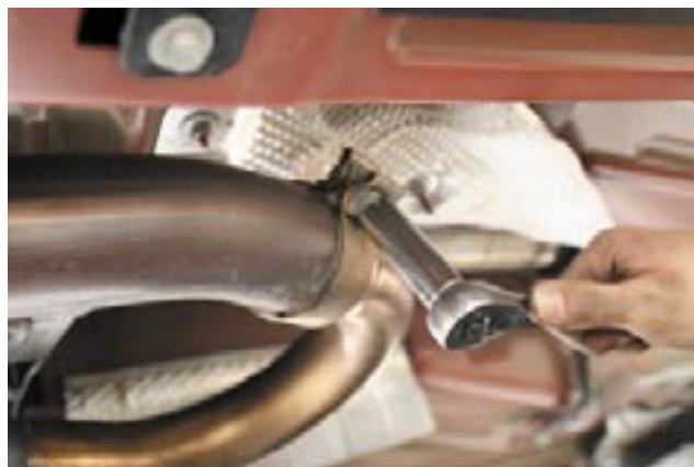
21. Install pipe HT 8 with supplied clamp on passenger side H pipe, leave clamp loose.
