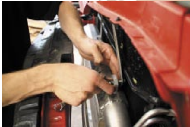
72. The long silicone hose will fit through the fender hole. The factory harness will need to be moved over to make room for the hose to push through. Enlarging the hole is an option, but not necessary.
