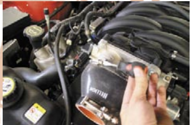
75. Install oval throttle body hose onto polished pipe and connect to throttle body.
