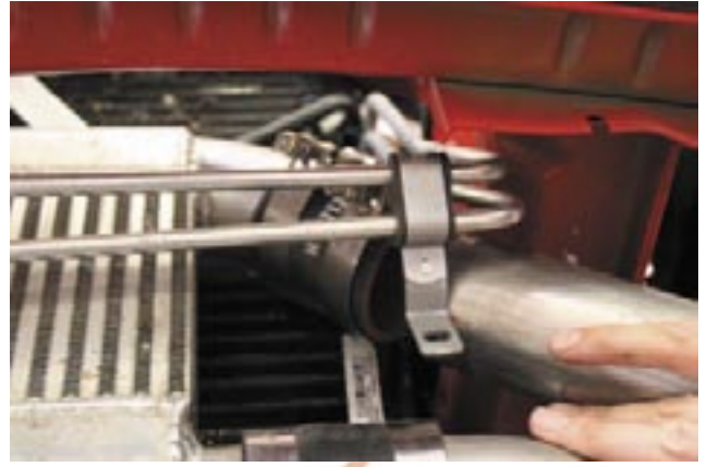
74. Push other side into intercooler and clamp.
