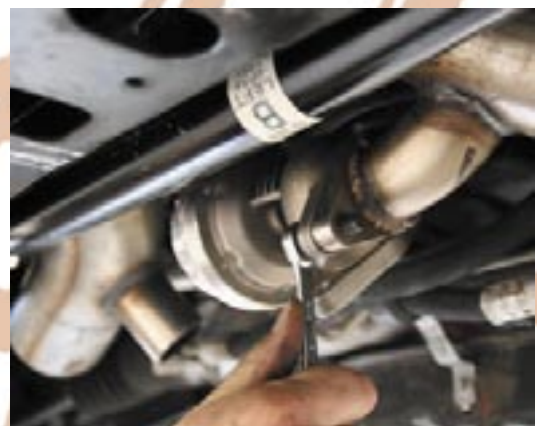
47. Slide HT 16 into wastegate re-entry bung and bolt to Wastegate using supplied bolts and gasket.
