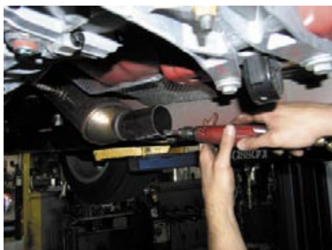
20. Install pipe HT 1 with supplied clamp on driver side H pipe, leave clamp loose.
