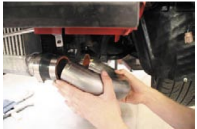
71. Next install the long 7 inch silicone hose over polished intercooler pipe 4 and secure with a clamp.
