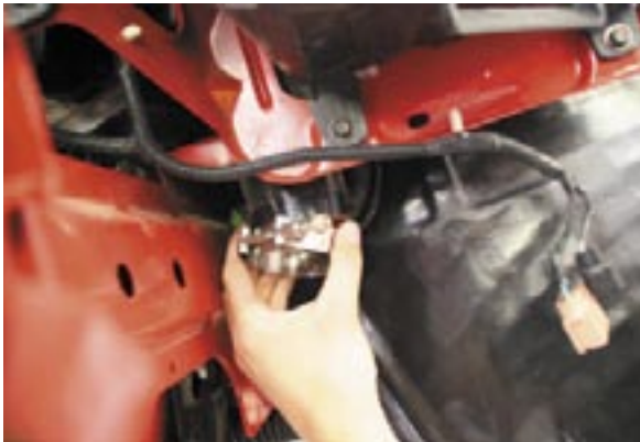
73. Next install intercooler pipe 3 (HT11) into long silicone hose and secure with clamp.
