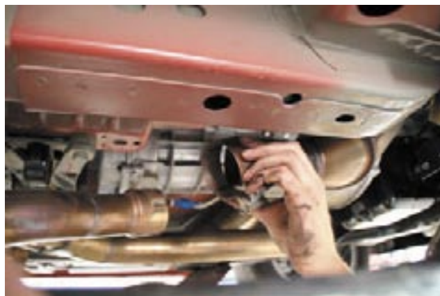
21. Install pipe HT 8 with supplied clamp on passenger side H pipe, leave clamp loose.
