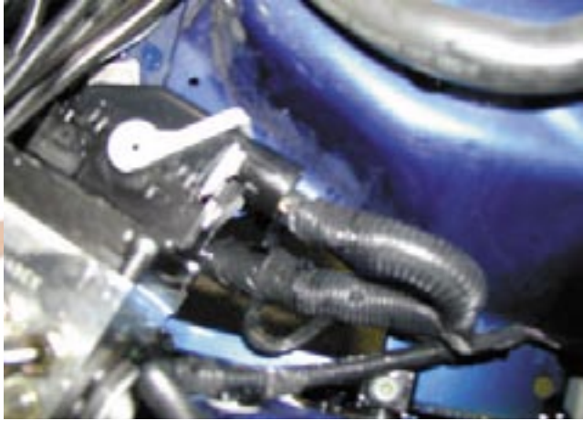
74. Push other side into intercooler and clamp.
