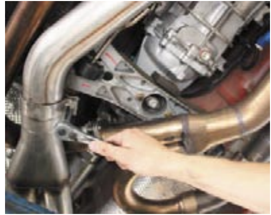
45. Put swaybar over studs and tighten nuts.
