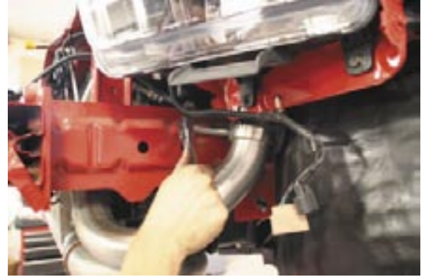
74. Push other side into intercooler and clamp.
