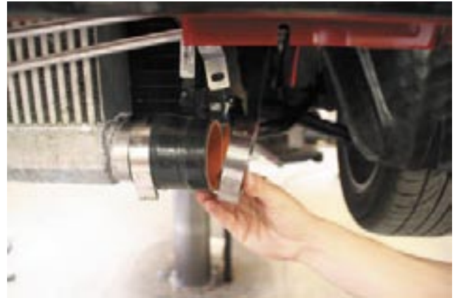
70. Install intercooler pipe 2 (HT10) with silicone hose and clamps onto intercooler inlet and onto intercooler pipe 1. (HT9)
