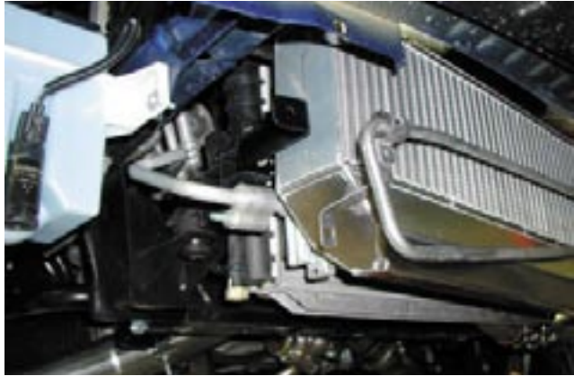
69. Bolt p/s line to supplied Z & U brackets using supplied 1/4" x 3/4" bolts, nuts and washers. Bolt brackets to factory location using factory bolts.
