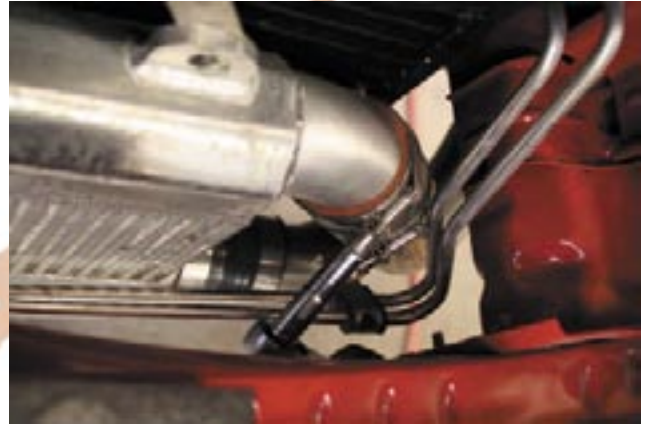
75. Install oval throttle body hose onto polished pipe and connect to throttle body.
