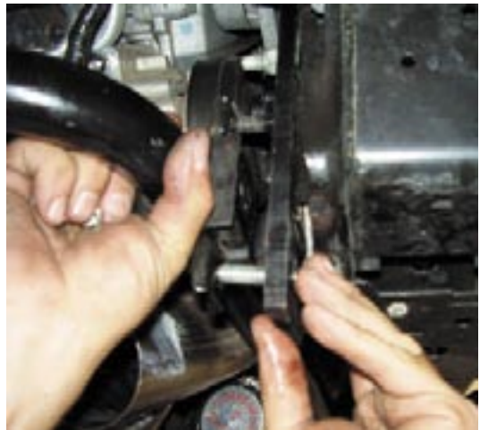
46. Install wastegate, using supplied bolts and nuts, There is no gasket between wastegate and HT 7.
