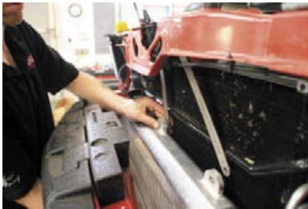
69. Bolt p/s line to supplied Z & U brackets using supplied 1/4" x 3/4" bolts, nuts and washers. Bolt brackets to factory location using factory bolts.
