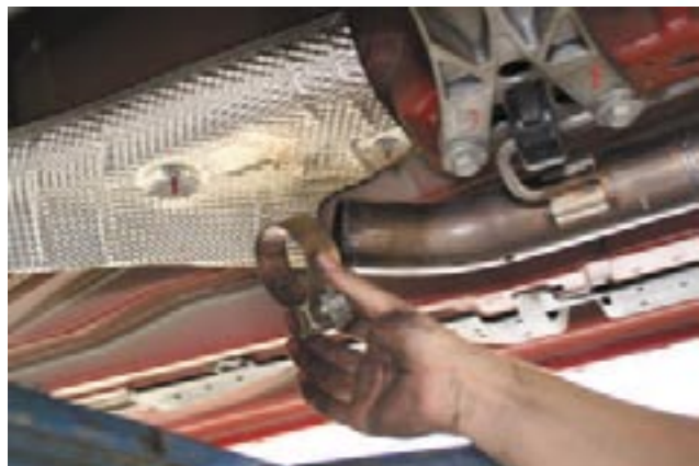
20. Install pipe HT 1 with supplied clamp on driver side H pipe, leave clamp loose.
