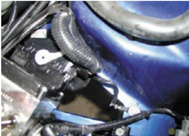
73. Next install intercooler pipe 3 (HT11) into long silicone hose and secure with clamp.
