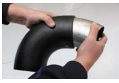
**72.** Ensure that hose stints are properly inserted into the middle of the 4" 90 degree rubber hoses.
