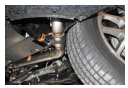
**81.** Next, insert Boost pipe #1 (Y-pipe) into both turbo compressors and into pipe #2. Leave clamps loose until desired fit is achieved. At this point, tighten all clamps and turbo housing bolts.
