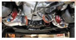
**71.** Next, install the steel air inlet pipes into the 4" Rubber 90 degree inlet hoses.
