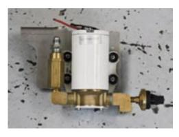
**35**. To install pump and bracket assembly, remove the front passenger nut that hold the right side of the k-member to the frame of the car. Position the assembly over the exposed stud and install the nut loosely.
