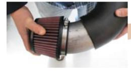
74. Next, install 4" rubber hoses with filters and inlets onto the turbocharger inlets. The hoses should be routed over the K-member and should place the filter at the pivot point of the A-arm. See photos for reference.
