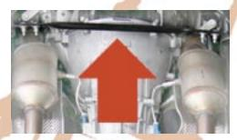
11. Install supplied 10mm bolts and washers through the "G-Trac brace" mounting holes. Bolts should go in from rear of vehicle with the threaded end towards the front of the car.
