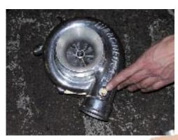
27. Using the metal gaskets supplied with turbo chargers, the 4 supplied 3/8"x 1" bolts, the 4 supplied 3/8" studs, and the 4 supplied 3/8" flange nuts - attach the turbo chargers to the up-pipes on their respective sides. (\*install the studs in the up-pipe holes closest to the *front* of the vehicle.)
