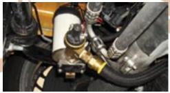
**41**. Remove the plastic line running from the super charger to the valve in the passenger side valve cover. Install the 2 supplied 5/8" vacuum caps with the  $\frac{1}{2}$ " hose clamps over the exposed barbs.
