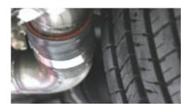
**88**. Locate <sup>3</sup>/<sub>4</sub>" Heat exchanger outlet hose, located near the front lip of the car, on the passenger side of the car. Clamp or drain the hose and cut as close to the middle as possible. See following picture to locate the hoses that you will be cutting.
