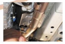
**18**. Loosely Install both up-pipes from exhaust manifolds on their respective sides using the factory nuts.
