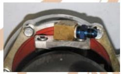
24. For the oil pressure feed side of the DRIVERS SIDE TURBO CHARGER: Install the supplied 1/8"NPT male to 1/8" female 45 degree fitting into the brass fitting already in turbo. Then install the brass oil check valve fitting (1/8"NPT male to -4AN male) into that 45 degree fitting.
