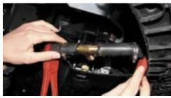
**90**. Locate the other hose, at the top of the engine, that runs from the factory intercooler to the coolant reservoir, and cut it as shown. After cutting, insert the other supplied <sup>3</sup>/<sub>4</sub> Tee and run the supplied <sup>3</sup>/<sub>4</sub> hose, with 1/8" worm clamps to the bottom fitting on the intercooler.
