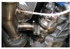
**67**. Install vacuum line supplied with waste gates from fitting in compressor housing to bottom side of waste gate (The non-polished side). If a boost controller will not be used, leave the port on the top side (polished) open to atmosphere.
