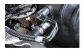
**42**. Unplug and remove the valve assembly from the passenger side valve cover. Use a piece of tape to temporarily seal exposed hole in valve cover. Using a ½" x 20 thread tap, tap existing two holes in valve cover. Clean debris out of holes and remove tape making sure not to get any metal debris in engine.
