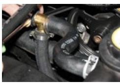
**91**. The intercooler system will need to operate for a while in order to bleed out any air that may be present in the system. Ensure that full coolant flow is established before attempting and dyno runs.
