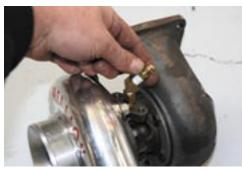
**26**. Install the 1/8"NPT male to 9/32" barb 90 degree fittings (Supplied with waste gates) into reference port in compressor housing (polished cover).
