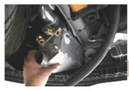
**86**. Install silicone hose on lower intercooler tank (with 3" T-bolt clamp on tank side), and insert small 45 degree tube. Leave clamps loose.
