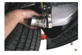
**87.** Attach 45\* tube to Boost Pipe #3 with steering wheel turned all the way to the right, and ensure that there is no interference. Tighten clamps.
