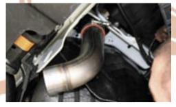
77. Next, install Bypass valve onto pipe #5, and then insert pipe #5 into the long silicone hose from pipe #4 that extends into engine compartment. Secure with clamp.
