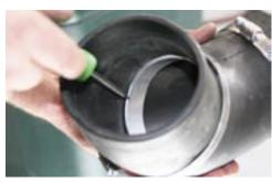
**73.** Now install supplied air filters onto the steel air inlets.
