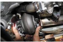
28. With turbo chargers tightened to up-pipes, install oil pressure feed lines to check valves on each turbo. Make sure that the oil feed and drain fittings are straight up and down, perpendicular to the ground for proper function.
