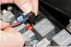
**49**. After installing fuse into holder, insert the mini add on circuit into the slot in the factory fuse block that you removed fuse #47 from.
