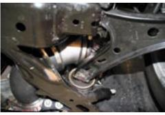
**75**. After Both elbows are installed, install Boost pipe #3 with T-bolt clamp and let it hang loosley.
