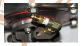
25. For the oil pressure feed side of the PASSENGER SIDE TURBO CHARGER: Install the supplied 1/8"NPT male to 1/8" female 45 degree fitting into the brass fitting already in turbo. Then install the oil check valve fitting (1/8"NPT male to -4AN male) into that 45 degree fitting.
