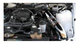
**80.** After all engine compartment pipes are connected, connect boost pipe #3 to the other pipes, and turn wheel to verify clearance. Leave clamps loose.
