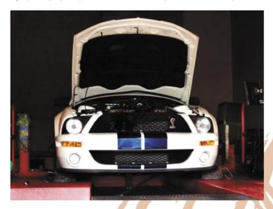
TAKE THE VEHICLE TO A DYNO FACILITY AMMEDIATELY AFTER INSTALL TO PREVENT ANY DAMAGE FROM OCCURING DUE TO THE TUNE. PUTTING THE VEHICLE UNDER BOOST WITHOUT THE PROPER TUNE MAY RESULT IN MAJOR ENGINE DAMAGE.
