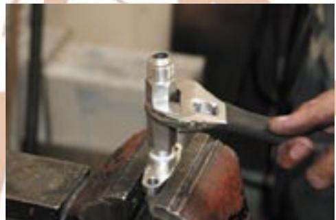
32. Loosen clocking bolts on turbocharger and install oil drain fitting and extension onto the turbo.
