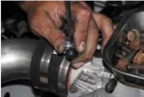
101. Install brass vacuum line fitting onto turbocharger compressor cover and tighten.
