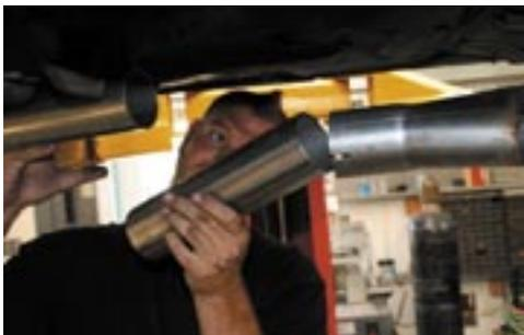
68. Next slide on 13" straight pipe using supplied clamp.
