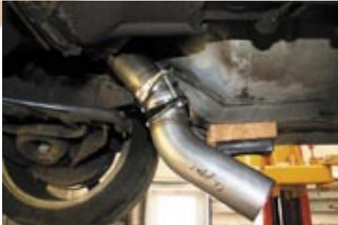
67. Slide either the 11" long straight pipe or catalytic converter over the downpipe extension, sliding 3" clamp first for easy installation.
