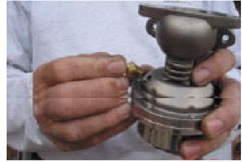
103. The rear cylinder head EGR ports will need to be plugged if smog crossover tube was removed (Non-emissions heads will not have to be plugged). To do this, cut the EGR tub about 1.5" from the point where it bolts to the head. Crimp this section and weld the end shut to prevent any pressure from escaping. Then attach to head at normal mounting point. (See image)
