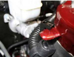
Use the supplied 1/4-20x1/2" bolt and attach JLT Bracket to the black mounting clamp using the smaller hole as shown below:
