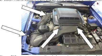
When installing a CAI you can remove the shaker system at the base of the Shaker scoop for a cleaner look. It has 2 clips on the top and 2 on the bottom that hold it on to the Shaker. Video shows this in detail.
