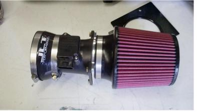
Put some tape around the hole in the apron. This will help prevent scratching the pipe during install. Bolt Apron Plate up using the stock air box bolt.
