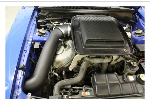
This kit includes an S&B Powerstack pre-oiled reusable air filter. The frequency you should clean your filter will depend on your driving conditions. It is recommended to check your filter at every oil change or 3,000 miles. If there is a build up of dirt as thick as the wire mesh, then it's time to clean your filter. As dirt builds up on your filter, the restriction of the airflow also increases. More frequent cleanings will improve your fuel economy and your vehicle's performance.
