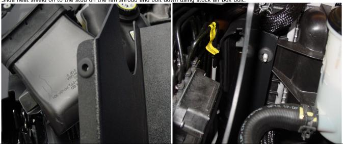
7 Unbolt the power steering reservoir and simply rotate the tank 180 degrees clockwise and install in the slot in the fan shroud and bolt back down using stock bolt.
