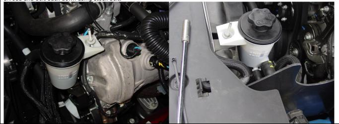
Remove the MAF sensor from the stock airbox using a trox T-20 driver and install in the JLT MAF housing using supplied Phillips head screws. Screws just need to be snug.
