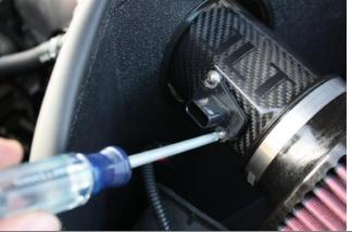
Plug in the MAF, PCV and automatic line (if used). Adjust tube for best fit and lightly snug all clamps.
