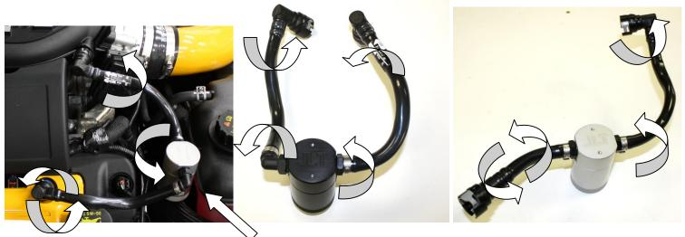
For BOSS manifold, raise hose and connect to fitting on manifold. Put wrench on angled fitting and rotate tank until it's level.
