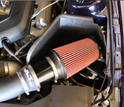
Oil Filter: The frequency you should clean your filter will depend on your driving conditions. It is recommended to check your filter at every oil change or 3,000 miles. If there is a build up of dirt as thick as the wire mesh, then it's time to clean your filter. As dirt builds up on your filter, the restriction of the airflow also increases. More frequent cleanings will improve your fuel economy and your vehicle's performance.
