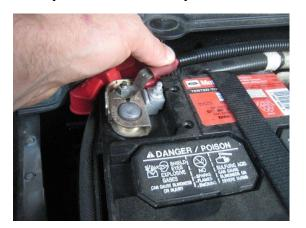
**2.** Press down on the positive cable end to bend down slightly.
