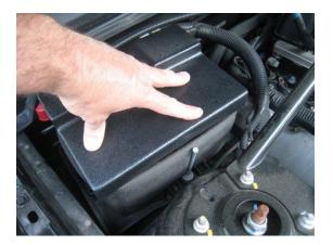
**5.** Remove the remaining backing from the Velcro and install Battery Cover by placing it over the battery and pressing firmly.
