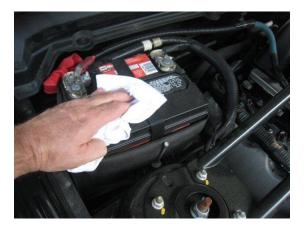
3. Clean the surface of the battery to remove any wax/grease/grime in order to ensure the best possible adhesion of the Velcro strips
