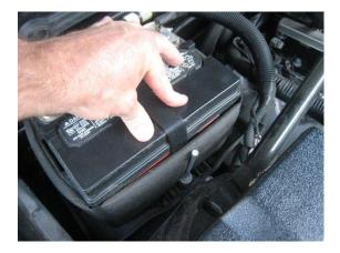
**4.** Remove the backing from one side of each Velcro pair and stick to the battery cover. Press firmly to ensure proper adhesion.
