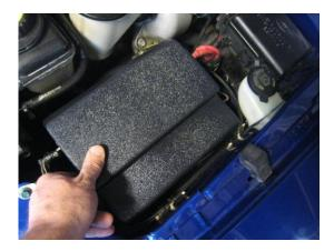
1. Test fit the battery cover; ensure that the battery cables fit through the access holes on the side of the cover.
