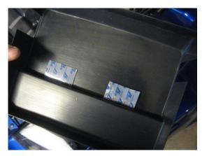
**4.** Remove the backing from one side of each Velcro pair and stick to the battery cover. Press firmly to ensure proper adhesion.
