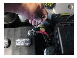
2. Loosen the battery cable(s) in case they need to be repositioned to fit through the access holes of the cover.
