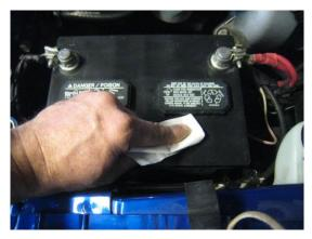
Clean the surface of the battery to remove any wax/grease/grime in order to ensure the best possible adhesion of the Velcro strips.
