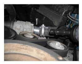
**STEP 11:** Install the new lower radiator hose onto the radiator and release the hose clamp.
