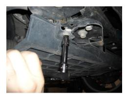
**STEP 18:** Reinstall under tray to front bumper cover with (9) bolts.
