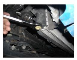
**STEP 5:** Remove (3) bolts securing the rearward underbody shield and lower.
