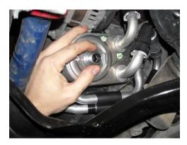
STEP 14: Tighten and torque the new threaded fitting to 58 Nm (43 lb-ft).
