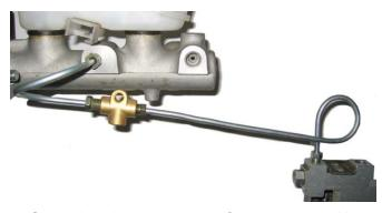
5. Gently bend the driver side front brake hard line towards the rear of the vehicle until it can be inserted into the remaining port of the Tee fitting.
