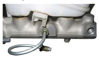
Connect the free ends of the brake hard lines installed in Steps 2 & 3 into the supplied Tee fitting. The remaining port of the Tee fitting should face down towards the ground.
