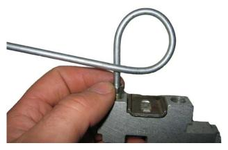
Thread the remaining 3/16" brake hard line with M10-1.0 bubble flare fittings into the rear port of the master cylinder. Position the free end of the brake hard line towards the front of the vehicle.
