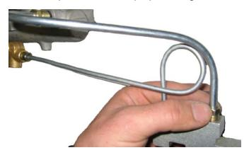
9. Thread the opposite end of the brake hard line installed in Step 8 into the forward port of the master cylinder.
