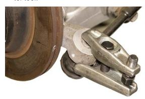
Note: If you have the MMIRSTR-1 or MMIRSTR-2 Adjustable IRS Tie-Rod Kit installed, it is not necessary to remove the tapered stud from the spindle. Simply unbolt the 5/8-18 Nylock Nut and remove the rod end from the tapered stud while taking note of the spacer stack arrangement for reinstallation purposes.
