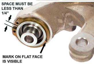
34. Repeat the process installing the three remaining MM Cross-Axis Joint. All four joints are oriented in the same direction; with the flange towards the front of the car.
