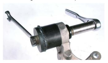
21. Repeat the process for the remaining cross-axis joints.
