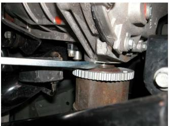
11. Pull the spindle/axle assembly out of the vehicle.
