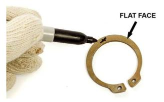
33. Using the supplied snap ring pliers, install the supplied snap ring into the groove on the MM Cross-Axis Joint, with the *FLAT* face of the snap ring facing *AWAY* from the spindle.
