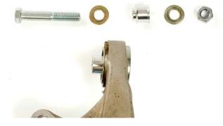
35. Place two greased washers under the 7/16-14 x 2-3/4 bolt head and pass the bolt through a preinstalled Bearing Insert.
