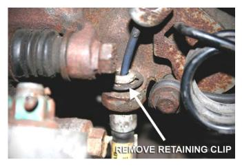
Disconnect the parking brake cable from the parking brake lever on the caliper, and remove the cable from the locating hole in the caliper.
