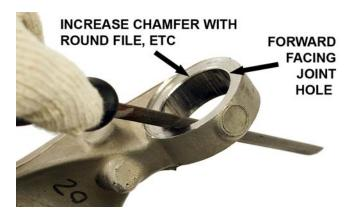
23. Apply a thin layer of the supplied Green Loctite to the inside diameter of the aluminum spindle's cross-axis joint hole, and to the minor outside diameter of the MM Cross-Axis Joint. The surfaces must be wiped clean of any grease prior to the application of Loctite. Brake cleaner or Acetone is recommended, but any non-water based cleaner will work.
