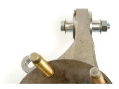
38. Draw the Bearing Insert into the spherical bearing by tightening the bolt with a pair of wrenches. Make sure the Insert seats flush against the face of the spherical bearing.
