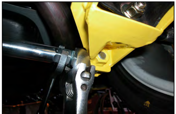
Incorrect- The rod ends are not aligned
