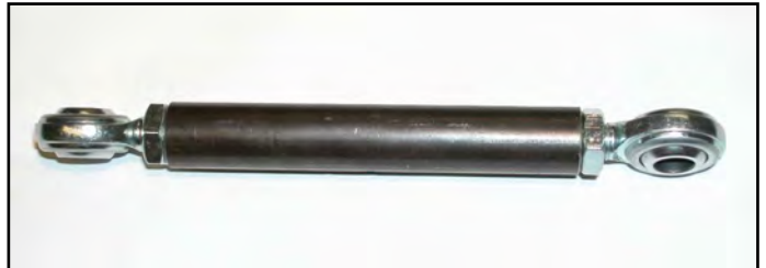
Incorrect- The rod ends are not aligned
