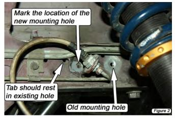
Move the brake line bracket out of the way and drill a 1/8" diameter hole on the mark made in Step 4. (Figure 3)
