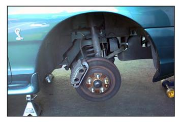
4. Unbolt the brake caliper and hang it securely. *Do not* let the caliper hang from the brake hose, as this can cause unseen damage to the hose. Steel braided hoses are especially susceptible to damage if the caliper is dropped or allowed to hang unsupported.
