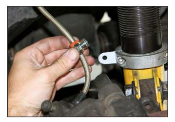
58. Pass the bolt through the Brake Hose Tab, place a washer onto the bolt, and secure the bolt with the nylock nut.
