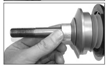
34. Place the 17mm inside diameter Thrust Washer over the top of the strut shaft. Do not be surprised if the Thrust Washer will not contact the shoulder of the shaft. The thick small diameter O-ring from Step 27 will be compressed and expanded during installation, Copyright © 2010 Maximum Motorsports, Inc. and the Thrust Washer will then contact the shoulder of the strut shaft.
