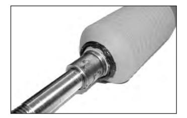
28. Place your 2-1/2" diameter Coil-Over Spring onto the Lower Spring Perch. Position the Lower Spring Perch so the top of the spring is below the top of the large-diameter portion of the strut shaft. That will keep the spring from interfering with the installation of the Upper Spring Perch Assembly.
