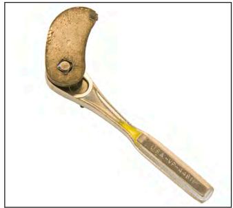
16. Fit the slotted end of the tool over the flange as shown. The flange can be bent by pushing down on the wrench. Reference the photo in the previous step to see where the tool needs to be used.
