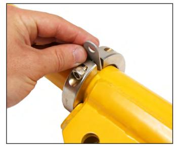
21. Position the Split Clamp Collar as low as possible so that it can clamp evenly on the strut housing. If you have MM Struts, the Split Clamp Collar will contact the top of the spindle mounting ears. If you have Bilstein Struts, the Split Clamp Collar will be in position when it contacts the top of the weld, preventing it from sliding down the strut housing.
