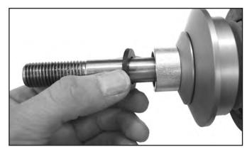
NOTE: Some companies' C/C plates have a fixed-type spacer bushing pressed into the spherical bearing. With these types of C/C plates, skip Step 35, and you may not be able to maximize bump travel in Step 38.
