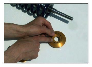
30. Place one Needle Bearing Race into the recess on the top side of the Upper Spring Perch. Completely pack the Thrust Needle Bearing with a high quality Moly wheel bearing grease. Place the Thrust Needle Bearing on top of the installed Needle Bearing Race. Place the second Needle Bearing Race on top of the Thrust Needle Bearing.
