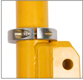
20. Remove the bolt from the rearward position of the Split Clamp Collar and insert the Brake Hose Tab as shown. Reinstall the bolt.
