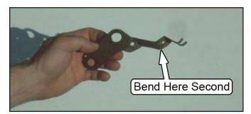
50. Reattach the mounting bracket to the spindle and adjust the bends if necessary to keep the mounting bracket close to the strut. Install and tighten the retaining nut for the mounting bracket.
