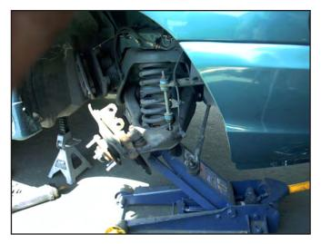
12. Carefully lower the control arm with the jack and remove the spring. If necessary, use a spring compressor. Often, aftermarket springs are shorter and can be gently "popped" out once the control arm is lowered far enough. Stock springs are quite long and require a spring compressor for safe removal.
