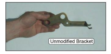
48. Use two sets of pliers to hold and bend the bracket forward near the base.
