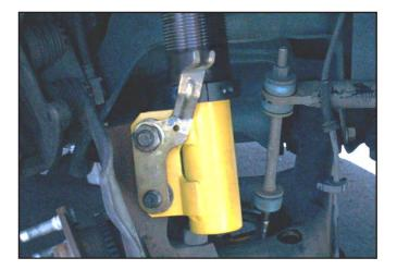
51. Clean any dirt from the tip of the ABS sensor and reattach the ABS sensor to the spindle. Reattach the sensor's wire to the mounting bracket.
