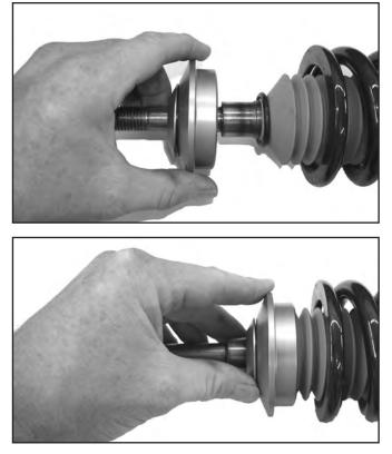
33. Slip the large 7/8" inside diameter Spacer Bushing over the strut shaft. It will sit down onto the Thrust Cone.
