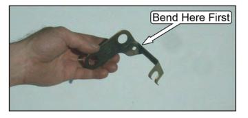
49. Then carefully bend it upward near the end where the wire attaches.
