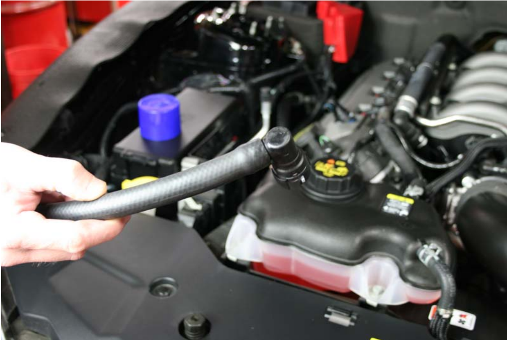
Step 8: Insert 90 degree fitting into one end of 1/2" hose
