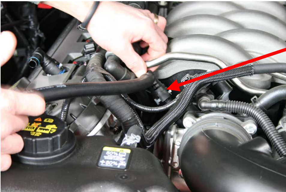
Step 9: Re-Install 90 degree fitting to intake
