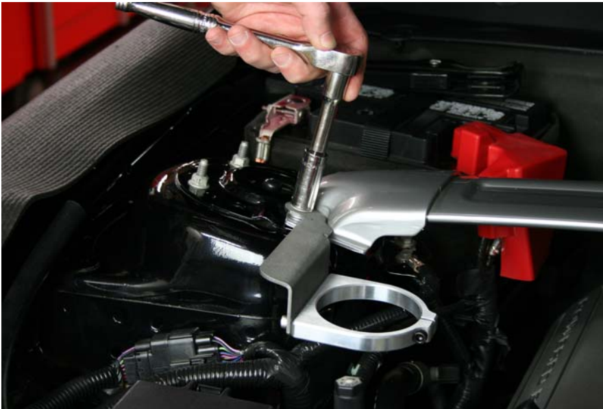
Step 13: Install Billet / Stainless mount to Strut Tower Brace
