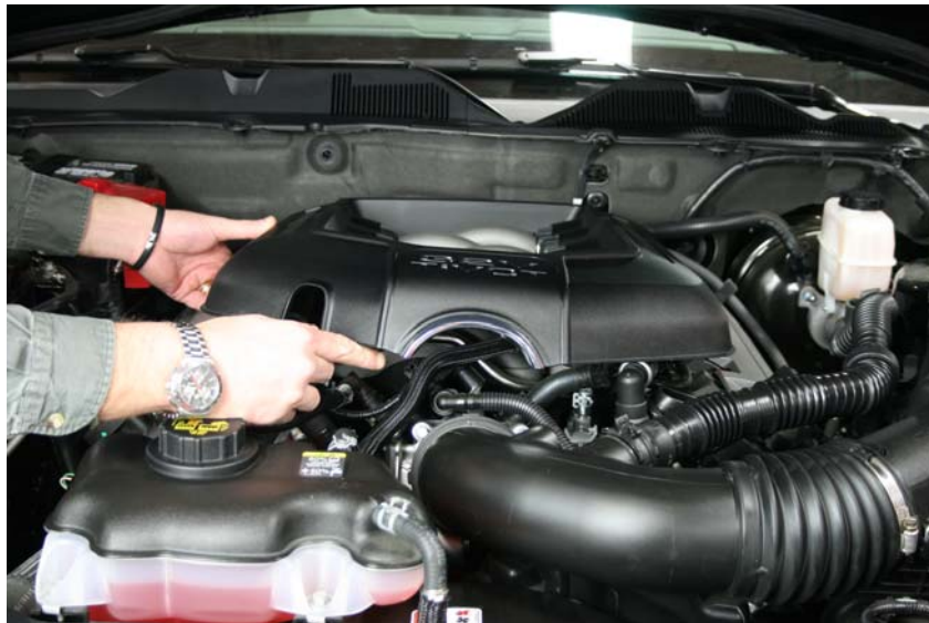
Step 2: Remove Intake Cover
