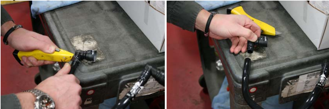
Step 4: Cut 90 degree fittings from PCV tube
