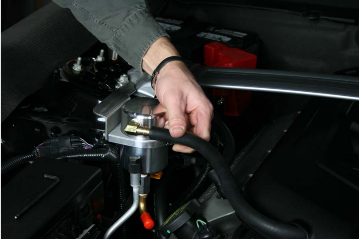
Step 24: Install to front 90 degree push lock fitting
