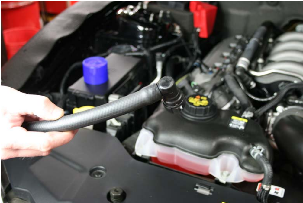
Step 18: Insert 90 degree fitting into one end of 1/2" hose
