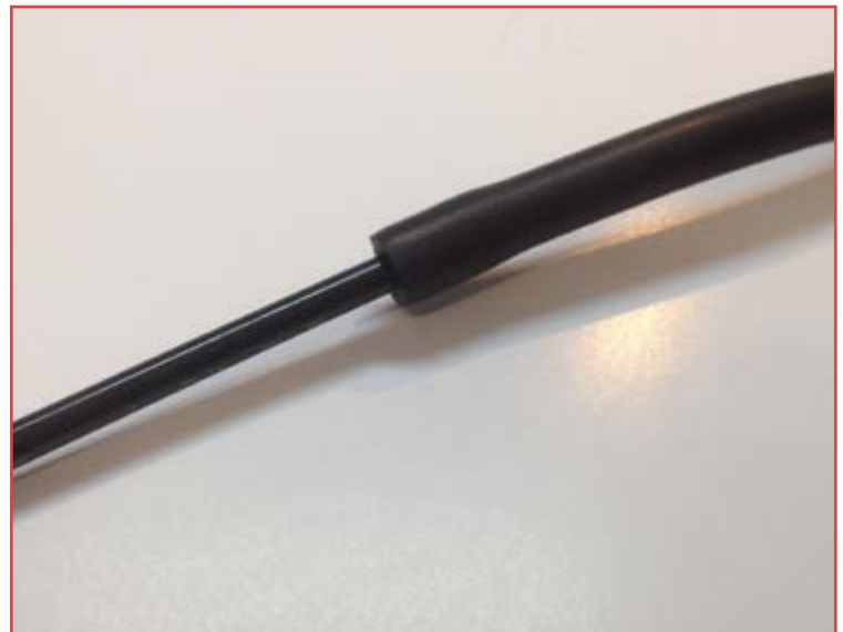
Use the wire Extension kit to extend the Red/White 10 gauge wires. Install the wire loom to protect the wires.
