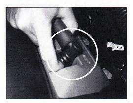
6. Remove the factory Ford coil cover by pulling up on it.
