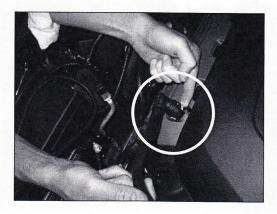
2. Remove the factory Ford coil cover by pulling up on it.
