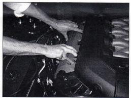
3. Install the RH side POWERED BY FORD or ROUSH coil cover by placing it over the ball studs on the cam cover & pushing down firmly to seat.
