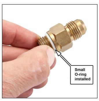
7. Install the Yellow fitting into the bottom inlet port of the steering rack. Torque it to 22 ft-lb.
