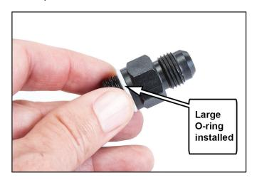
4. Lightly coat the threads of the fitting with the supplied hydraulic sealant. To prevent the sealant from getting into the fluid system, DO NOT coat the leading thread on the fitting.
