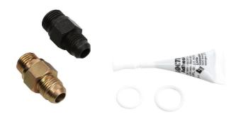
3. Install the larger of the two PTFE O-rings over the rack side (the end that threads into the steering rack) of the supplied Black adapter fitting. It is necessary to carefully stretch the PTFE O-ring somewhat and rotate it down the threads until it seats up against the shoulder of the fitting.
