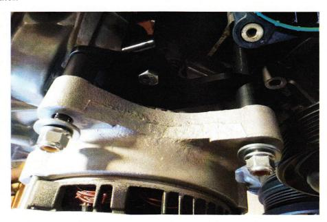
14. a. If using a 1996-2001 Cobra alternator you will need to install the small "L" bracket with 8mm and 6mm bolt provided.
