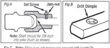
Fig C Note: Make sure set screws are secured with Loctite™ thread locker and shaft is dimpled, and inspect periodically.
