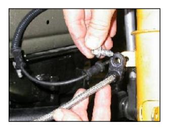
Each stainless steel front brake line for the Mustang GT is pre-fitted with a new line locator.
