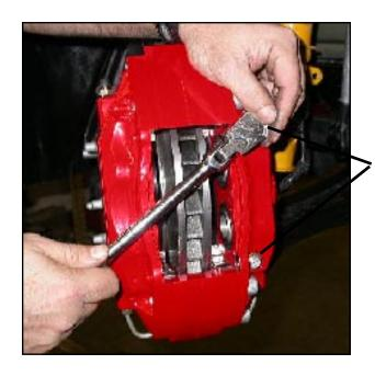
Install the Jet nuts onto each stud, with one 12mm washer under each nut. Tighten the Jet nuts to 40 lb-ft of torque, using a 1/2" socket.
