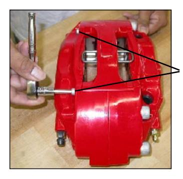
Remove the two bolts holding the caliper bridge in place, using a 5mm Allen wrench.
