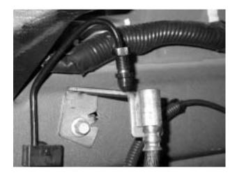
Remove the hard line fitting, and place one of the rubber caps over the end of the hard line, to control fluid loss during the installation.
