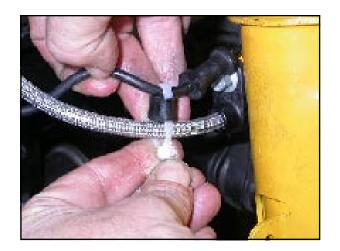
After securing the brake line, turn the wheels lock-to-lock, to ensure that the brake line is not binding in any way, nor interfering with any suspension component, including the CV boot and axle/drive shaft.
