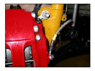
The orientation of the banjo fitting should be as shown in the photograph, with the brake line angled toward the strut bracket.
