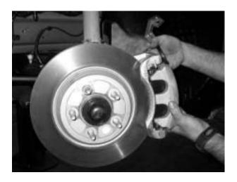
Remove the caliper with the stock brake line attached. There may be some leakage from the open end of the brake line, especially if the pads/pistons on the caliper are retracted.
