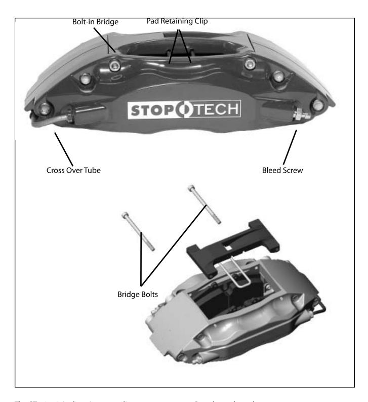
The ST-40 original equipment caliper uses a common Porsche-style pad. The Friction Materials Standards Institute (FMSI) number for the pad backing plate is D609.
