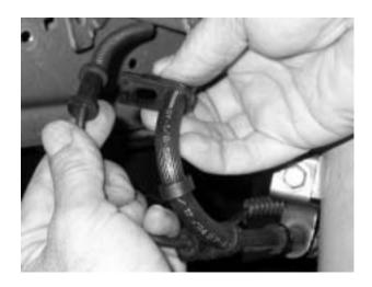
Separate the ABS lead from the stock brake line by releasing it from the two plastic clips which are fixed to the stock brake line.
