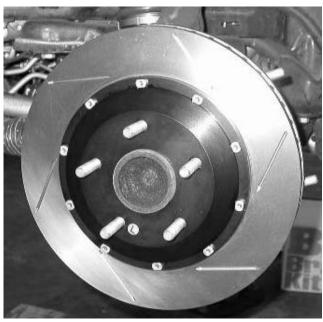
Note: Be sure that the rotor assembly is on the correct side of the car, as reversing the rotors will severely decrease the cooling capacity of the system. The rotors are clearly marked "L" and "R" with orange tags on the rotor hats. If the tags are not legible, the vanes inside the rotor should lean to the rear of the car on the top side of the rotor (see the following pages for more-detailed images).
