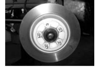
The dust shield must be permanently removed from each front wheel of the Mustang GT, to accommodate the AeroRotor.
