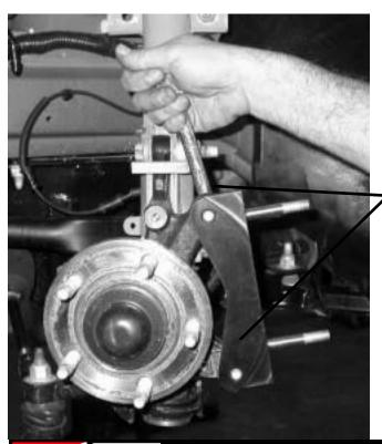
Remove the Jet nuts and washers from the caliper mounting bracket, and put them in a safe place for later use.
