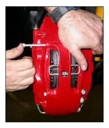
Insert the first bridge bolt, from the outside of the caliper, and start the first few threads, using a 5mm Allen wrench.
