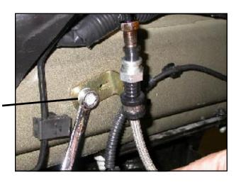
Remove the rubber cap from the hard line, and screw the stainless steel brake line onto the hard line fitting by hand for a few turns. It may be necessary to remove the bracket, in order to start the threads. If so, snug the two fittings together, and reinstall the bracket, taking care to ensure that all connections are tightened, using the wrenches shown on the following page.
