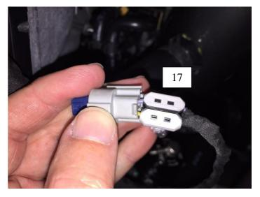
18. Secure the OEM BOV solenoid plug with the scotch locks by using cable ties. As shown.
