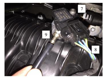
Route the vacuum hose towards the left hand side of the engine towards the factory BOV location. (Bottom left hand side of engine when facing the vehicle.)
