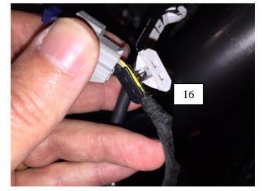
17. The scotch locks should look like this when installed correctly. Scotch locks are removable if the factory BOV is to be re-installed.
