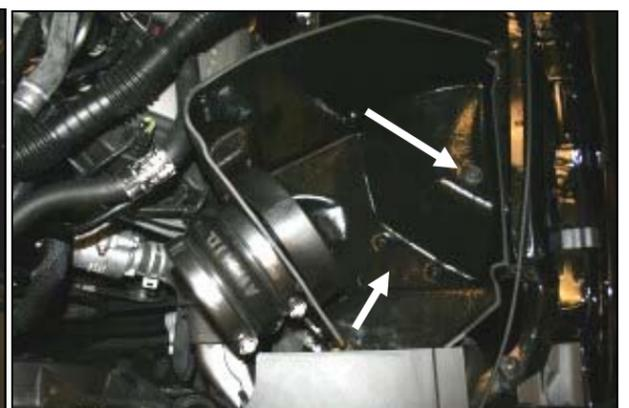
9. Install the CAB into the vehicle. Make sure that the Air inlet of the CAB aligns with the factory duct, and the two locating pins on the bottom align with the factory grommets. Next reinstall the factory bolt that was removed in step #3 thru the steel sleeve and grommet and into the inner fender.
