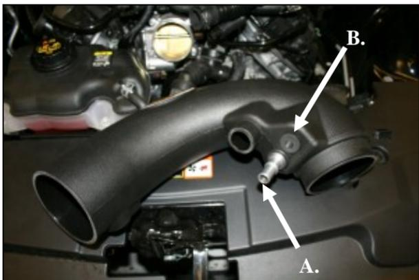
4. Install the Grommets and Fittings into the Airaid intake tube (#2). A) All models will require the use of the 5/8" Fitting (#19) and the 5/8" Grommet (#20). B) Automatic transmission equipped vehicles will also use the 3/8" Fitting (#18) and 3/8" Grommet (#21). Manual transmission vehicles will not need the 3/8" components and will use the Blind Grommet (#22).
