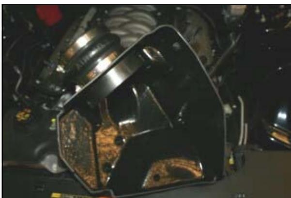
8. Install the hump hose (#5) onto the filter adapter using two #72 hose clamps (#13) as shown. Leave the two hose clamps loose for now. Transfer the Resonator stand off from the factory air box into the CAB.
