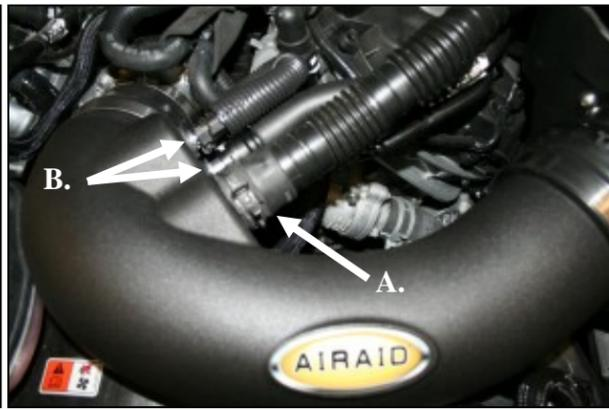
11. Install the Airaid Intake Tube into the couplers as shown, and tighten all Hose clamps. **A)** Reconnect the Resonator tube to the Airaid Intake using the OEM clamp. **B)** Reconnect the breather line/lines to the Aluminum Fittings depending on your application.
