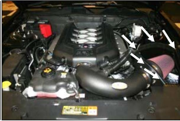
14. Install the Weather Strip (#9) onto the CAB with the contoured edge going away from the filter. Start at the front of the vehicle and work your way back. Replace the engine cover.
