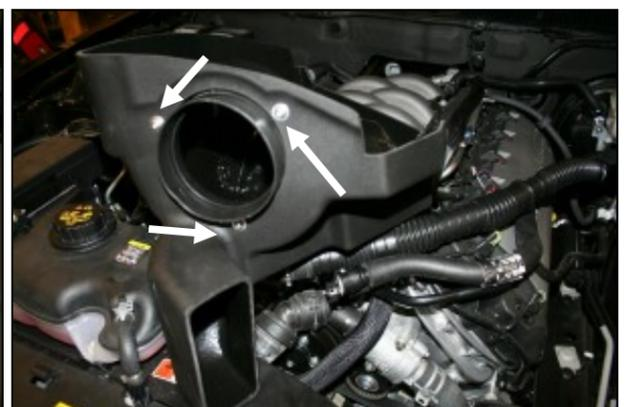
6. Install the filter adapter (#8) using three 1/4-20 button head bolts (#10), and flat washers (#11) into the Airaid Cool Air Box (CAB) (#4) as shown.
