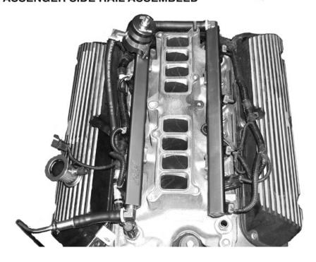
KIT INSTALLED WITH OPTIONAL REGULATOR SHOWN
