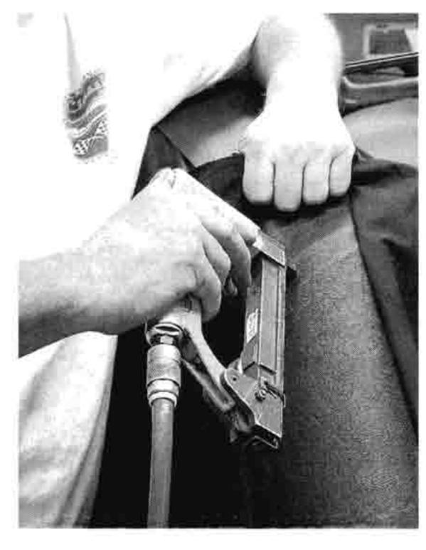
16 As with the main pads, the quarter pads are stapled to the top frame with an air-powered stapler after trimming and final adjustment.
