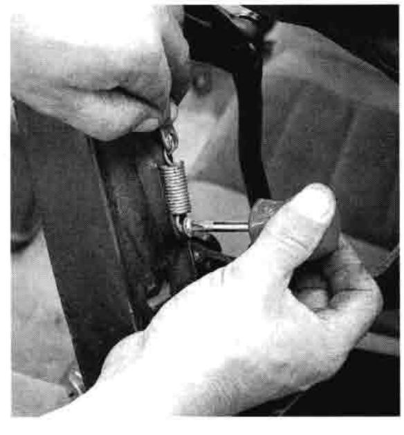
6 Towards the rear of the top, the old cables are removed by unscrewing these springs. As with the clips shown in the previous photo, the springs are also reused with the new cables.
