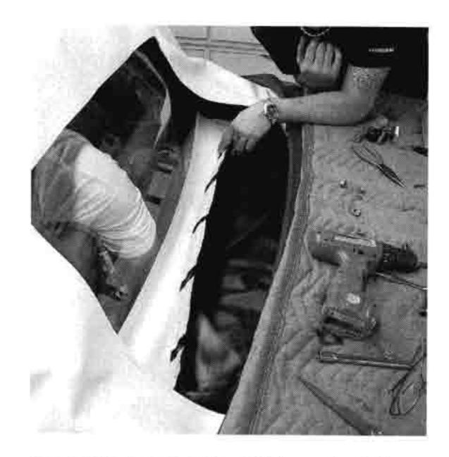
23 This is one of the trickier parts of the installation. The rear quarter pads (shown in step 15), the window, and the top canvas are all installed at the same time at the back of the car. They are also all connected to the staple bar. Once attached, most of the remaining installation is at the front half of the top.
