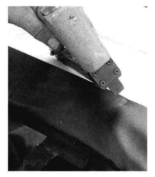
14 Once the pads are sized and fitted, they're stapled into place on the bows that run across the top frame.
