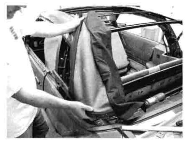
15 Next, the rear quarter pads are testfitted and installed. They run from the top bow above the rear window and attach to the car at the rear staple bar.
