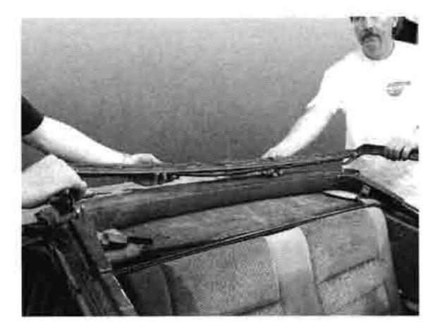
3 Once all the screws are removed, the windshield can be lifted up and removed from the car.
