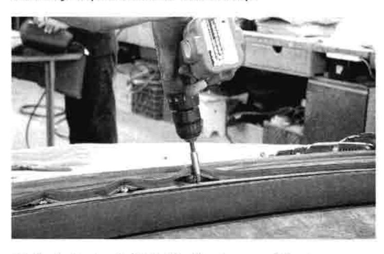
2 Next, the top is folded in the down position to access and remove the weatherstrip that seals the elements at the top of the windshield. Although these can be replaced, they are removed carefully so the weatherstrip can be reused with the new top.
