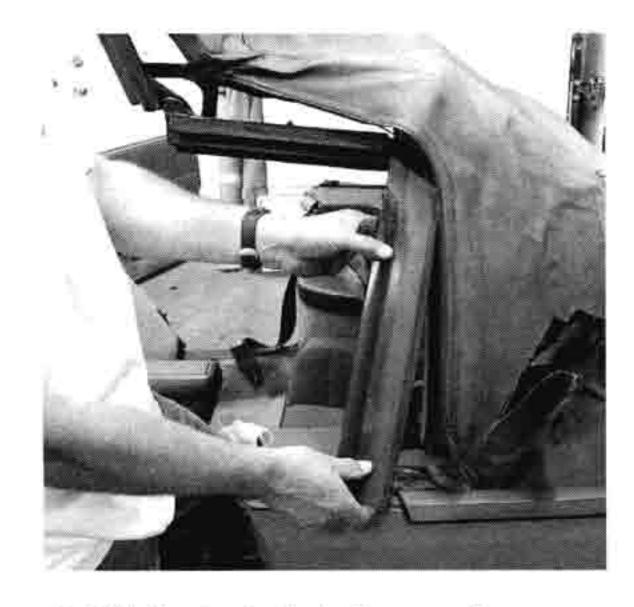
With the top in the halfway position (between fully lowered and raised), these retaining bars need to be removed. The two bolts that hold them to the top (one bar on each side) are accessed from inside the car while sitting in the back seat. These pieces are saved and reinstalled with the new top.
