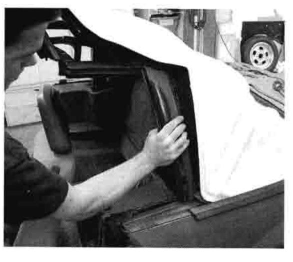
25 The retaining bars (shown being removed in step four) are reinstalled after the top is glued into place underneath where they mount to the frame. The top is fully attached where it joins the car.
