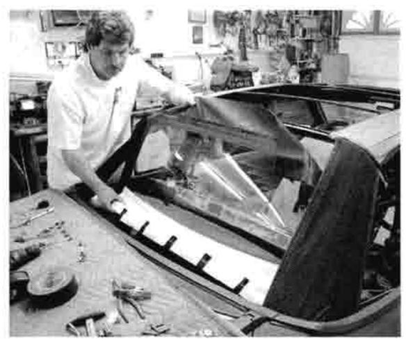
17 As shown here, the top frame has its full complement of pads already installed on both sides. For the most part, the pads are stapled into place. Upholstery adhesive is used in some places, as well. Size up and fit the glass rear window next, which Mike is doing here. The window has already been installed onto the main rear staple bar, which attaches to the car in the top well, just in front of the trunk lid.
