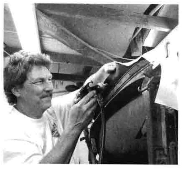
24 Back at the front of the top frame, the top is glued into place after it's trimmed and final-fitted. Once glued, it's finally secured into place by reinstalling the weatherstrip that was removed to access and remove the old top canvas.
