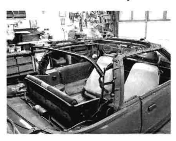
12 Here's the bare top frame almost ready to accept the new top canvas, pads, cables, and glass rear window. But first it is thoroughly cleaned with a rag and some cleaner. Glass cleaners like Windex or kitchen cleaner like Formula 409 work well. If you desire, the frame can also be repainted.
