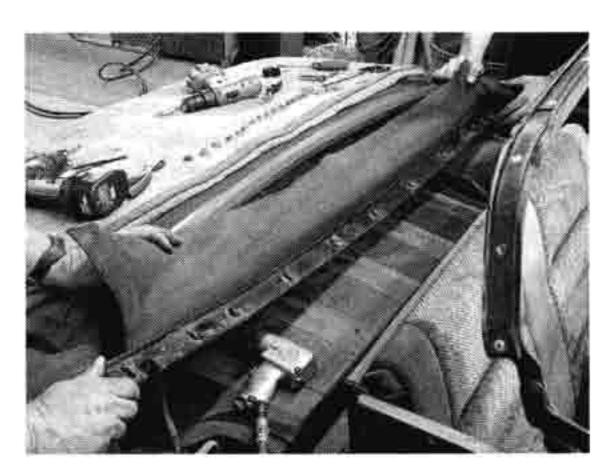
10 Once unbolted, the staple bar (or well frame) is removed along with the remnants of the old top. Once out of the car, the staple bar is further disassembled to remove any remaining parts of the old top.
