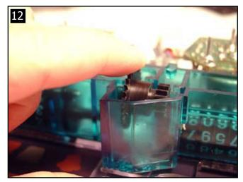
13. Using a flat blade screwdriver, begin prying off the drive gear. Once it is about half way off the shaft, you can finish removing it by hand.
