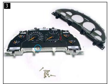
3. With the lens removed from the cluster, remove the single T15 torx screw below the speedometer.
