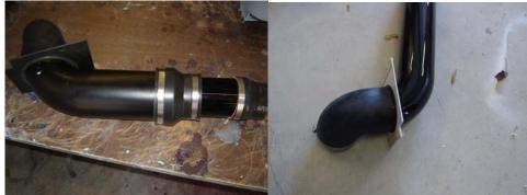
**NOTE:** The reducing elbow is a very tight fit. To ease this, use soapy water and/or heat it in the microwave for about 20 seconds. This will make it easier to stretch over the pipe. Also remember it will need to be at an angle like the photo above. So it may help to set the pipe and elbow in the car a few times to get the correct angle. Position the clamps so you can get to them once installed in the fender well.
