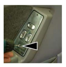
4. Using a 7/64 drill bit and drill, drill a ½" deep pilot hole for the bottom mounting screw. Using the supplied Phillips screw, fasten the bottom of the plate.
