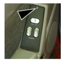
1. Remove the factory retaining screw on existing windows plates.
